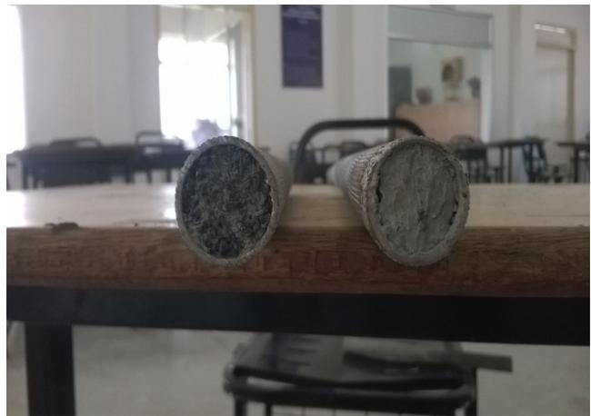
Fig. 2: Hollow mild steel pipe filled with rubber cement slurry
