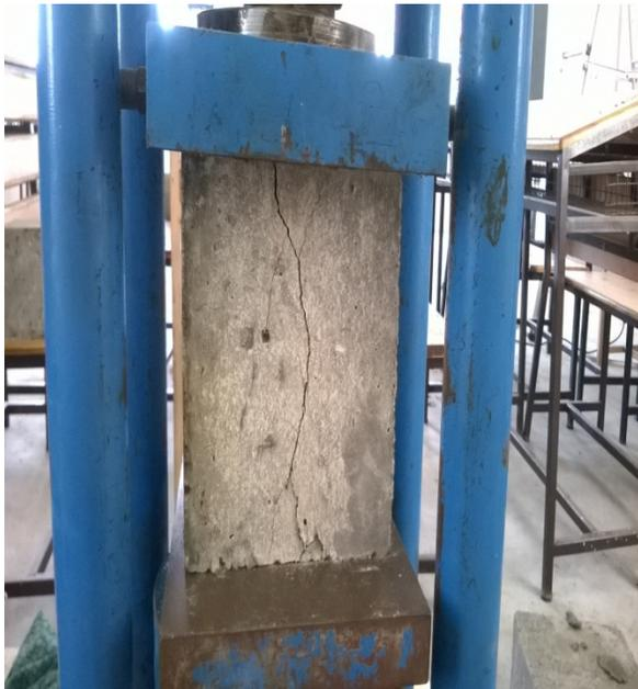
Fig 1: Initial cracking occurred during compression test after 28 days of curing
